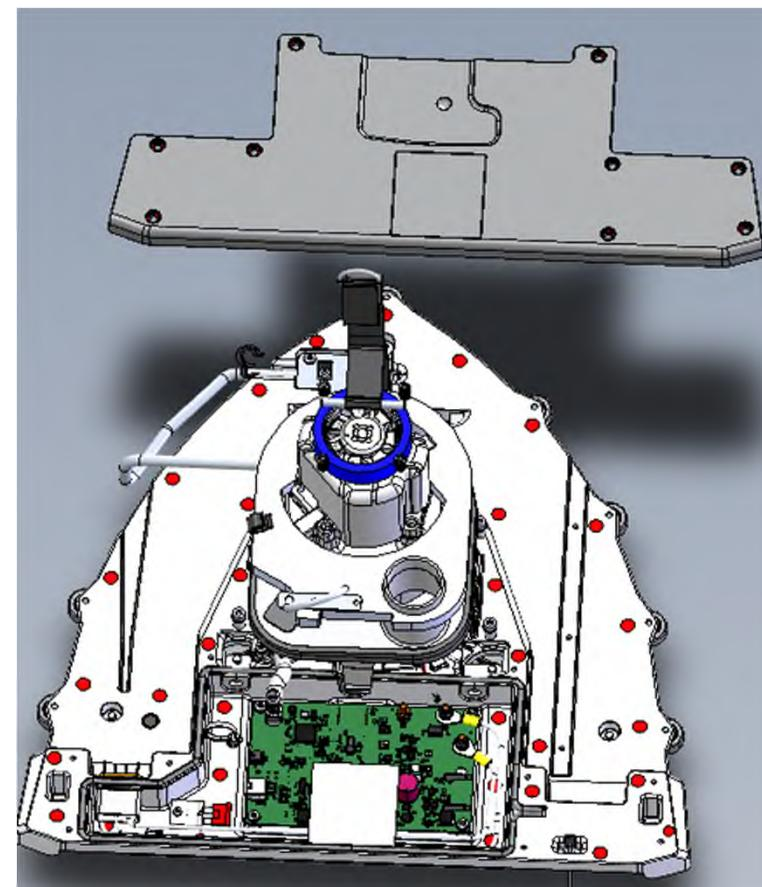
When assembling, pay attention to the cable and housing seal properly seated in the housing
