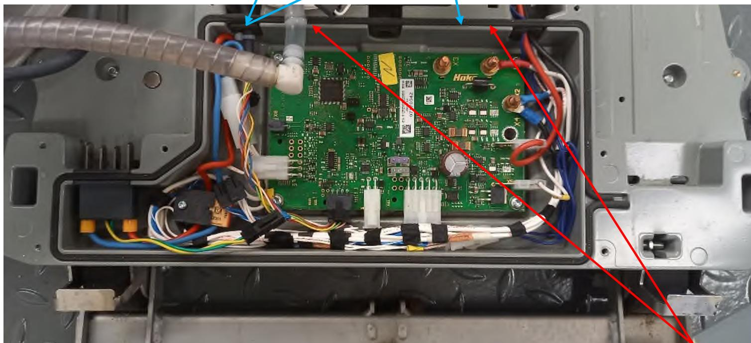
The housing seal is partially glued in. When replacing, fix again with Loctide 422 in two places
